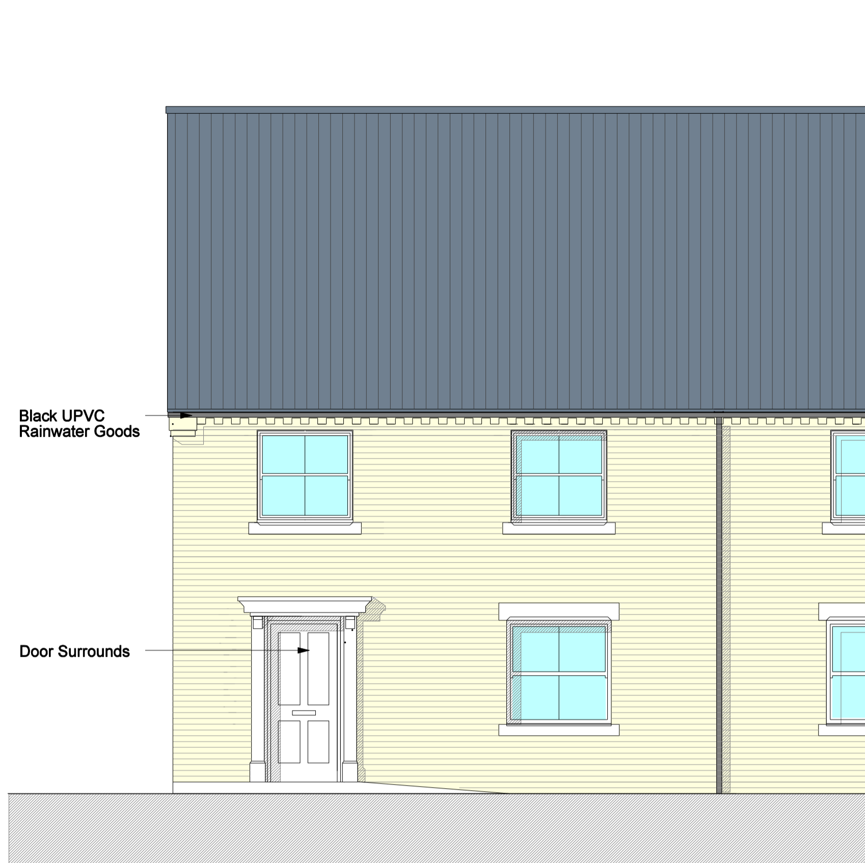
Front Elevation - End Terrace
