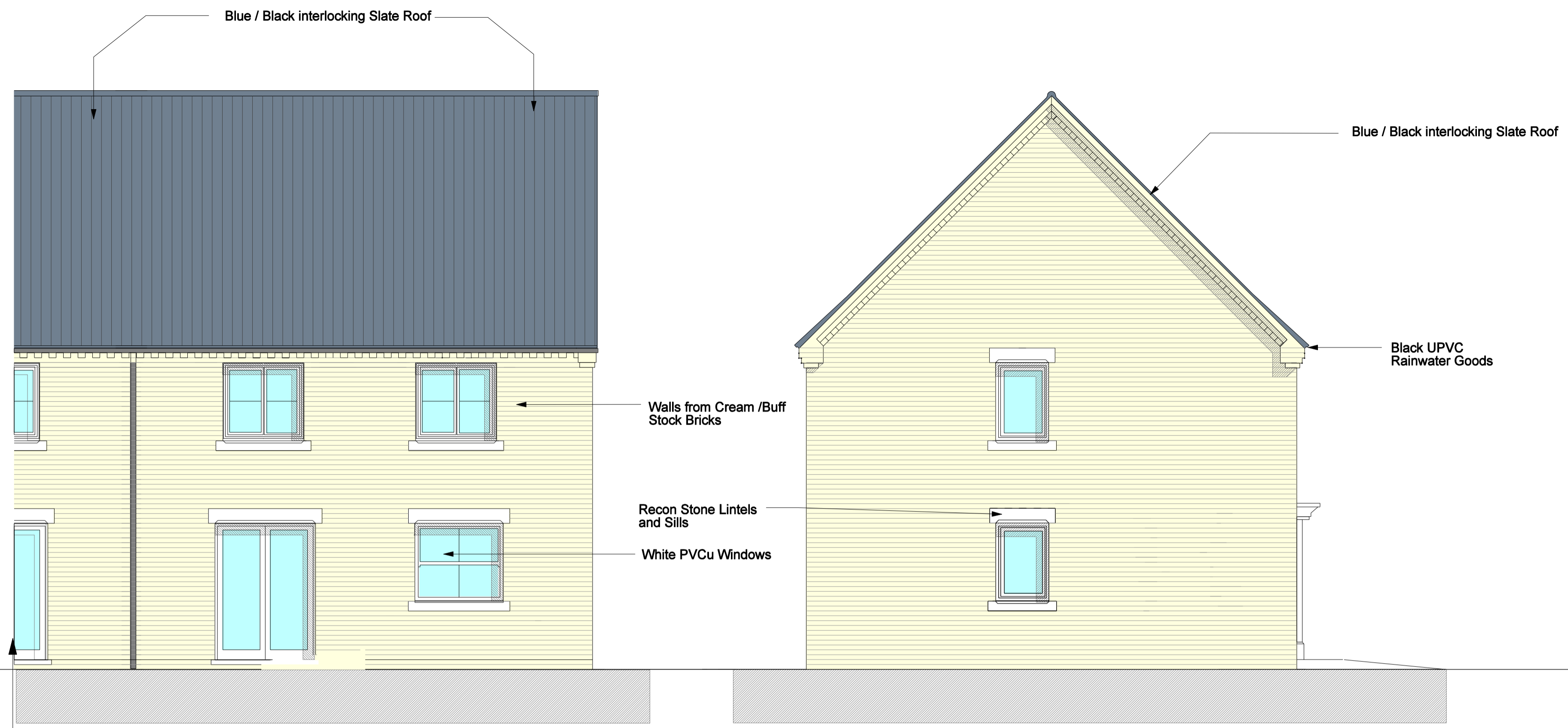
Rear Elevation - End Terrace
