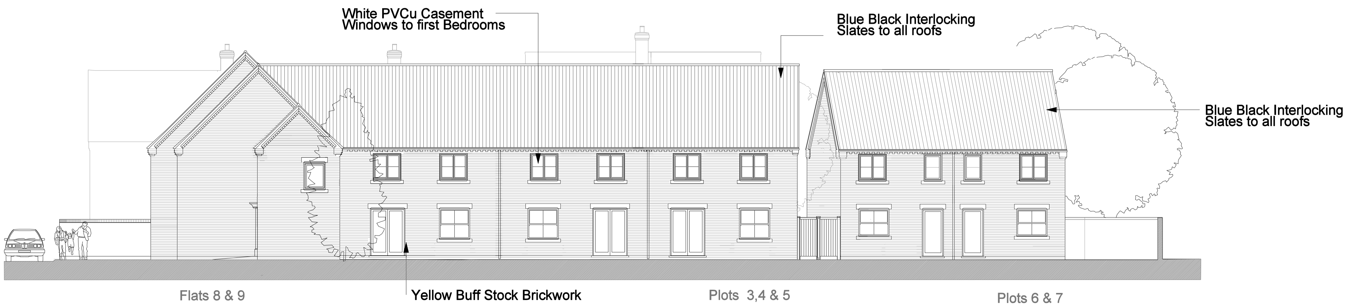
Internal Elevation C - C
