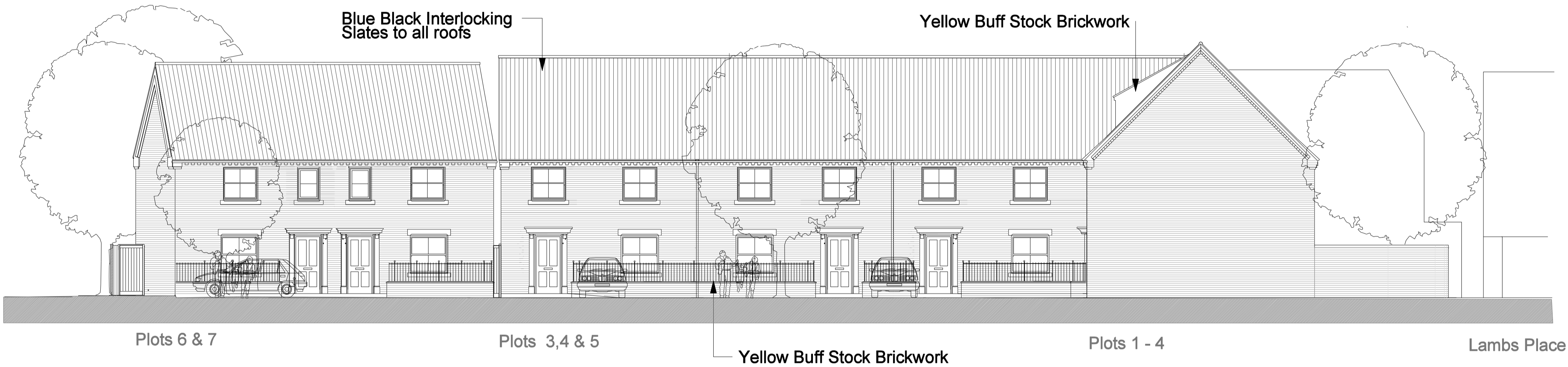
Internal Elevation B - B
